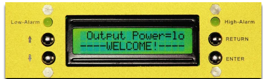
Repeater not receiving a good input signal
