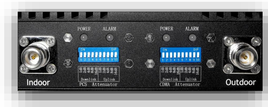
Example of Dual Band Repeater Dip Switches
