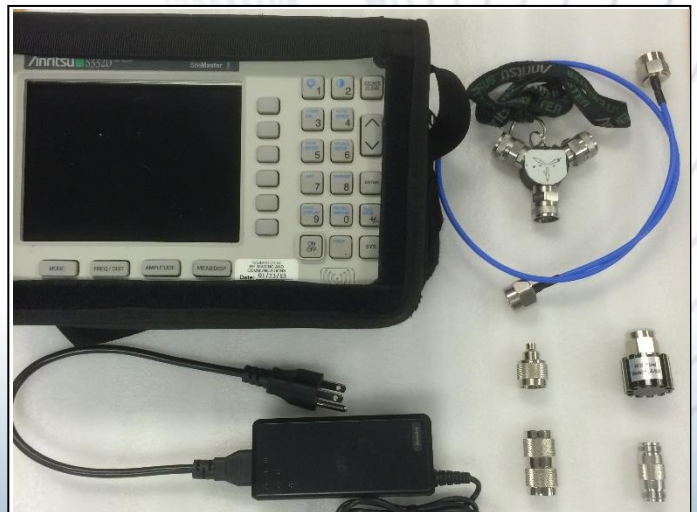
Use test equipment to verify return loss benchmark. >20dB
